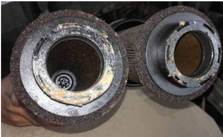
Soap formation due to presence of non ferrous metal
